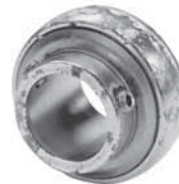
Zinc Plated Insert After Accelerated Corrosion Resistant Test
